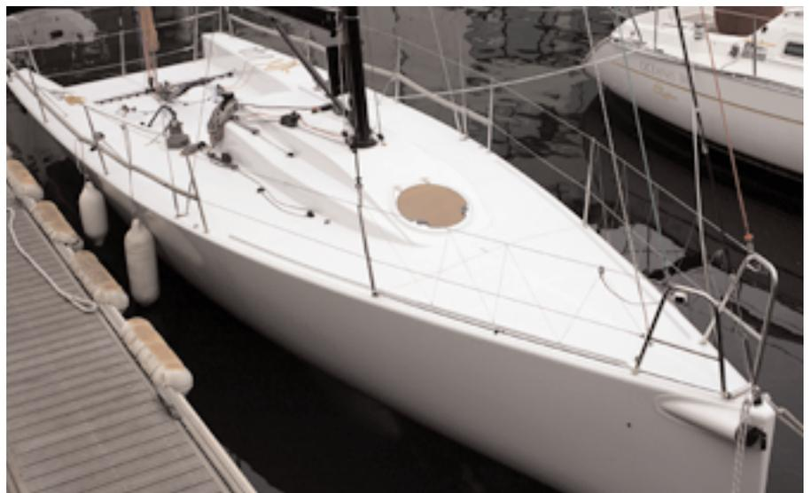
There is only one winch on the cabin top, the bow hatch is a simple composite fabrication with no aluminum frame and a pair of simple tackles with rings control the jib sheeting. There are no headsail tracks.
