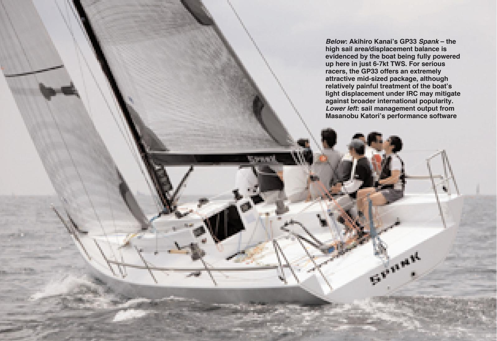
**Below:** Akihiro Kanai's GP33 *Spank* – the high sail area/displacement balance is evidenced by the boat being fully powered up here in just 6-7kt TWS. For serious racers, the GP33 offers an extremely attractive mid-sized package, although relatively painful treatment of the boat's light displacement under IRC may mitigate against broader international popularity. **Lower left:** sail management output from Masanobu Katori's performance software
